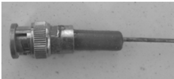
Figure 5: A close up of the quarter wave whip.
