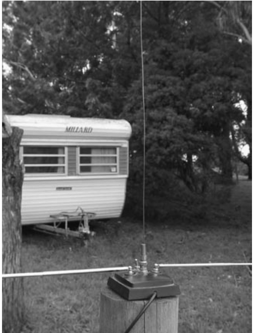
Figure 1: The set up in the field for FM or SSB use on 2 m. This antenna has been used in three states and 15 countries (as G3ZDR/p) with great results.
